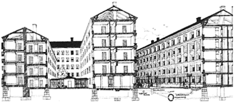
Figure 22.5 Stockholm. Section of a block at the end of the nineteenth century (drawing by the Stockholm town-building office). The approved town plans indicated only the location of the streets and the shape of the blocks; the height and basic design of the houses, the size of the courtyards and so on were regulated by the 1874 building ordinances.
