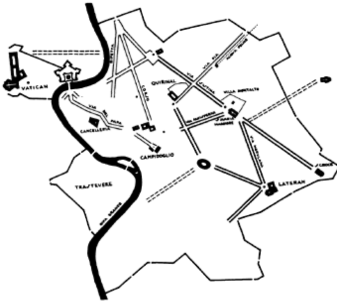
Figure 2.14 Following the final return of the popes to Rome in 1420, extensive regulation and expansion plans soon began to be considered. Street planning was set seriously in motion during the second half of the century, and was aimed in a first phase at facilitating communications in the densely built-up area in the Campus Martius and between this and the Vatican. In the 1580s under Sixtus V, planning embarked on a second and more wide-ranging phase, and a system of completely straight streets was planned by the pope and his architect Domenico Fontana, as communicating links between the great titular churches. The figure shows the streets planned by Sixtus (dashed lines=streets not realized). The pope's project differs from earlier planning in its grand scale and in the fact that the new streets were to serve primarily as traffic routes. A similar focus also characterises many nineteenth-century projects, above all Haussmann's transformation of Paris. Common to both is the desire to enliven long street prospects with focal accents. [From Magnuson (1982)]
