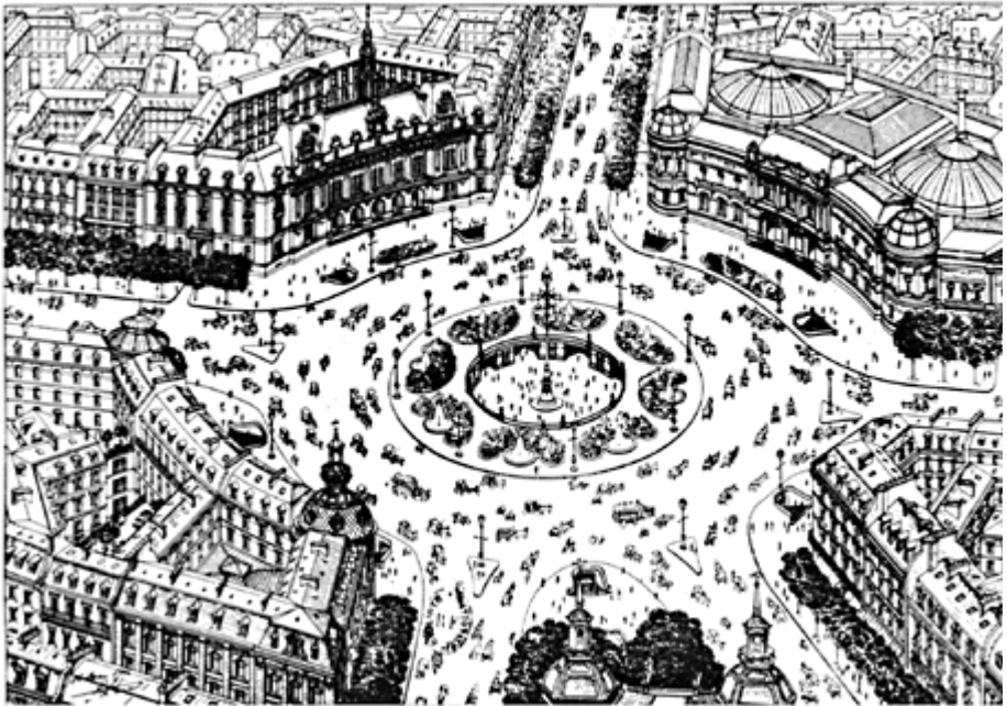
Figure 21.2 Eugène Hénard's pioneering proposal for a Carrefour a giration , 1906, used at the Place de l'Étoile since 1907. Until then there had been no rules for how to behave at cross-roads, which meant that conditions were chaotic at the major traffic junctions. It should be noted that Hénard also intended a lower level for pedestrians with various facilities; as we know, such arrangements became a recurring element in twentieth-century street planning, although pedestrians were seldom given the open space in the middle of the square, as Hénard envisaged. Among his many other ideas is a proposal for split-level crossings. [From Evenson (1979)]
